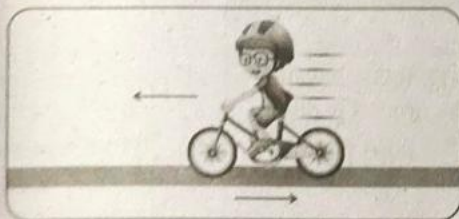
Frictional force stops the moving bicycle
